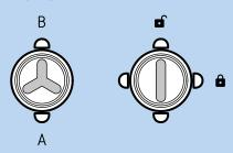
One can check the current position of the valve on the actuator. On the left the indicator of the 3-way valve (in position "B"). On the right the indicator on a 2-way valve (in position "open").
