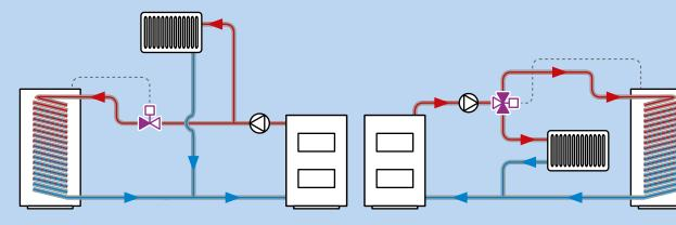
Above a system with domestic water heating priority. If the temperature in the tank decreases, the thermostat opens the 2-way **AZV** valve, so the boiler heats the tank rapidly. When the temperature in the tank is reached, the thermostat will close the valve.
