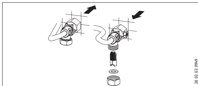
If contaminated, clean the strainer in the threaded cold water fitting. Close the shut-off valve in the cold water inlet line before removing, cleaning and refitting the strainer.
