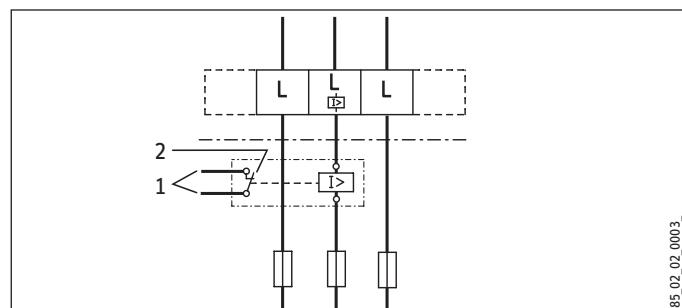
1 Control cable to the contactor of the 2nd appliance (e.g. electric storage heater).
